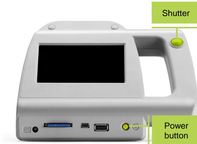
Figure 1: “plusoptiX A12R” rear side with touchscreen
