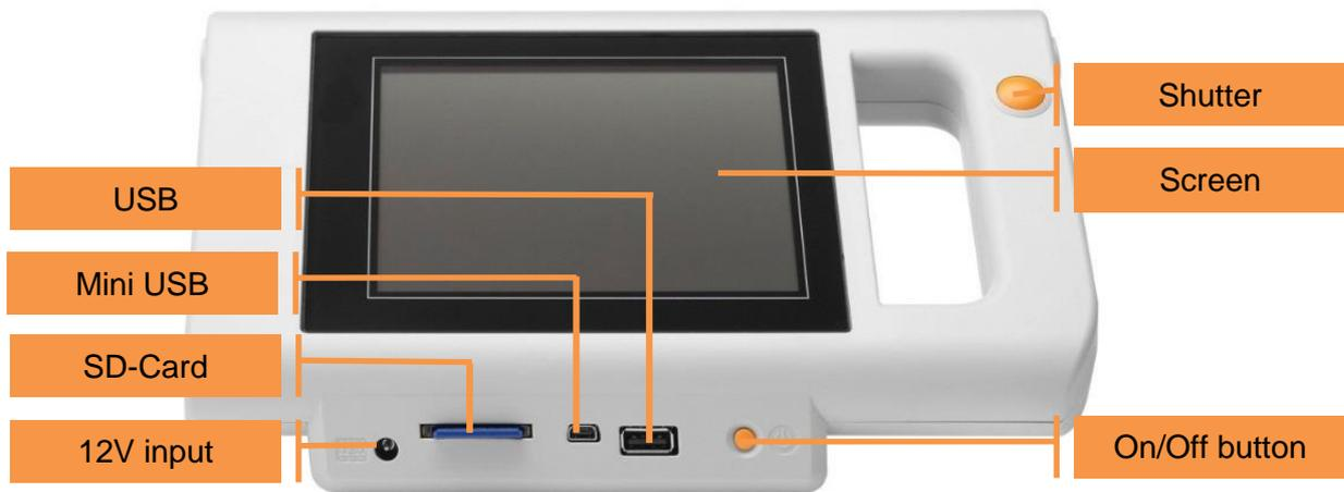
Figure 2: Rear view of the device
